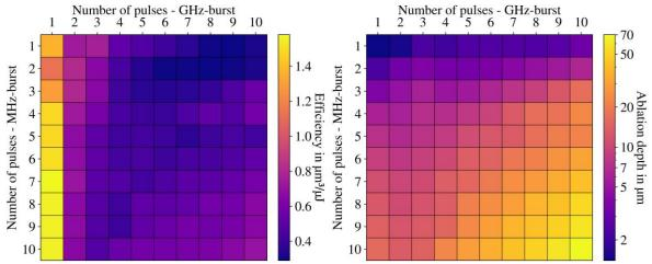
Efficiency and ablation depth with different burst parameters, a fluence of  $0.5 \text{ J/cm}^2$  per burst pulse and 5 passes.
