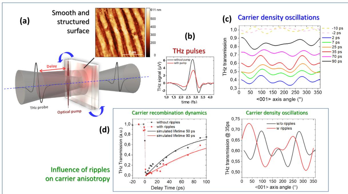
Figure 1: (a) Schematic of the measurement concept. (b) THz pulses used for probing the charge carrier dynamics. (c) Charge carrier density (THz transmission) oscillation with crystal orientation as a function of time. (d) Comparison of carrier density dynamics (left) and oscillation with crystal orientation (right), without (dark lines and dots) and in presence (red lines and dots) of LIPSS.
