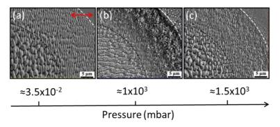
SEM micrographs of surface spots generated in (a) dry vacuum (b) air and (c) high nitrogen pressure, for 240 number laser pulses at a pulse energy of  $\approx$  170 µJ. The red arrows indicate the polarization direction.
