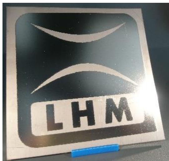
Figure 1: photograph of a partially laser polished surface, demonstrating the increased reflectivity of the polished area in comparison to the initial matte surface.
