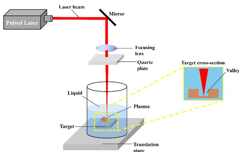
Figure 1 Schematic of experimental setup for valley ablation. the cross-sectional view of valley ablation target is shown (inset).
