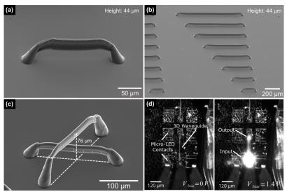
Figure 1. 3D Printed Polymer Waveguides. (a) A 44  $\mu$ m high and 200  $\mu$ m long 3D waveguide, with a rectangular core size of 9x33  $\mu$ m<sup>2</sup>. Printing parameters: zig-zag period T=1  $\mu$ m, laser fluence F=16.5 mJ cm<sup>-2</sup> for the waveguide core and F=19.8 mJ cm<sup>-2</sup> for the tapers, v=100  $\mu$ m s<sup>-1</sup>. (b) Side view of fabricated waveguides with height 44  $\mu$ m, with lengths ranging from 200 to 900  $\mu$ m.
